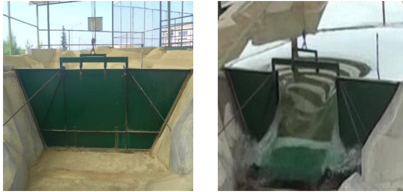
Figure 4. Simulation of the sudden failure of the dam
