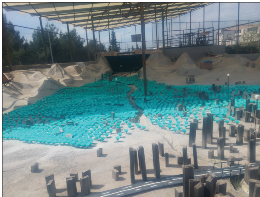
Figure 2. Physical model of Ürkmez Dam lake and downstream region with vegetation
