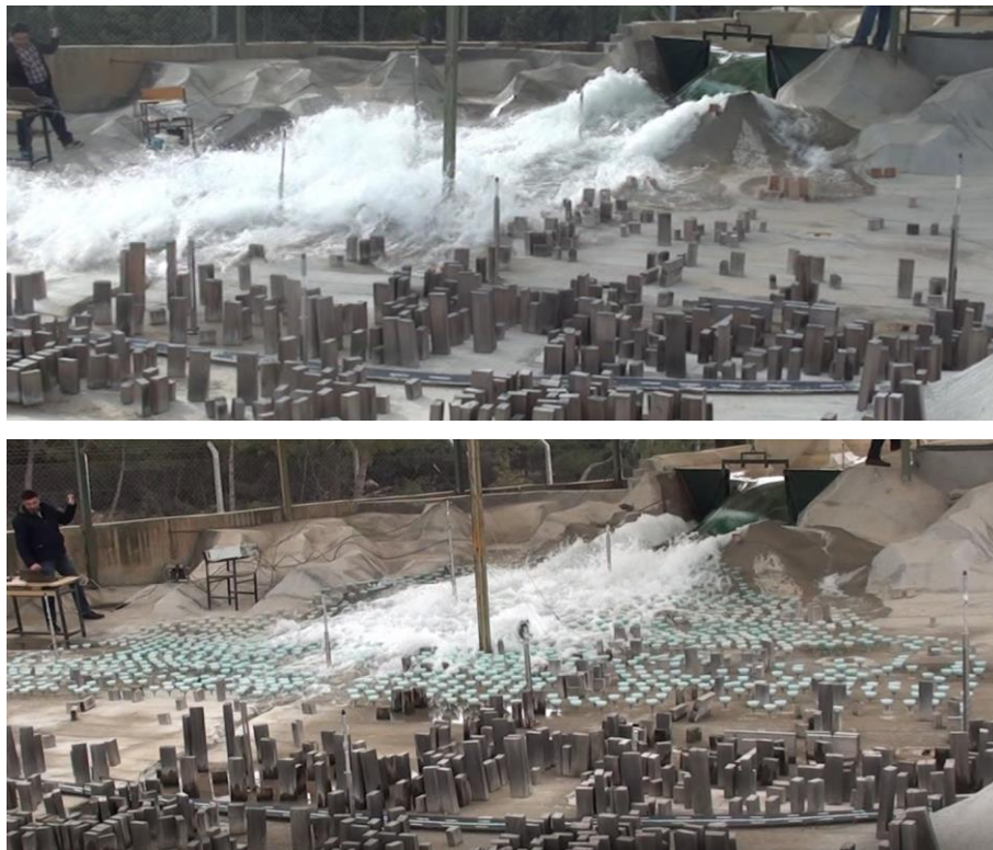
Figure 14. The regions that flood wave reached at time 3 s
