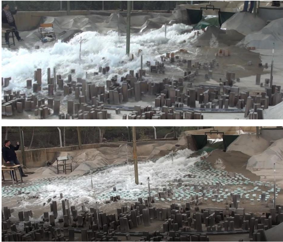
Figure 15. The regions that flood wave reached at time 6 s
