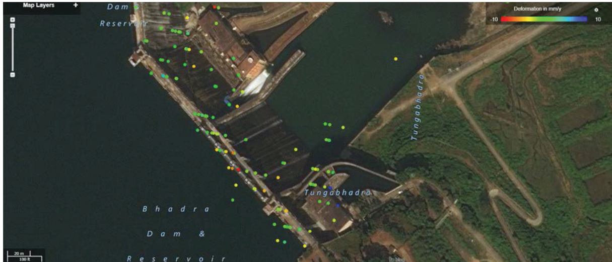
Figure 5. Main dam deformation (period 29 September 2016 to 11 March 2018)
