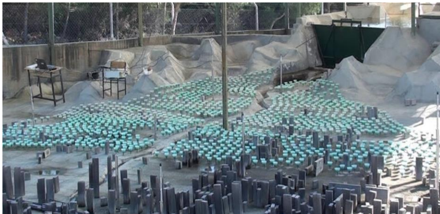
Figure 3. Distorted physical model of the Urkmez dam involving its reservoir and downstream part with partial plant configuration
