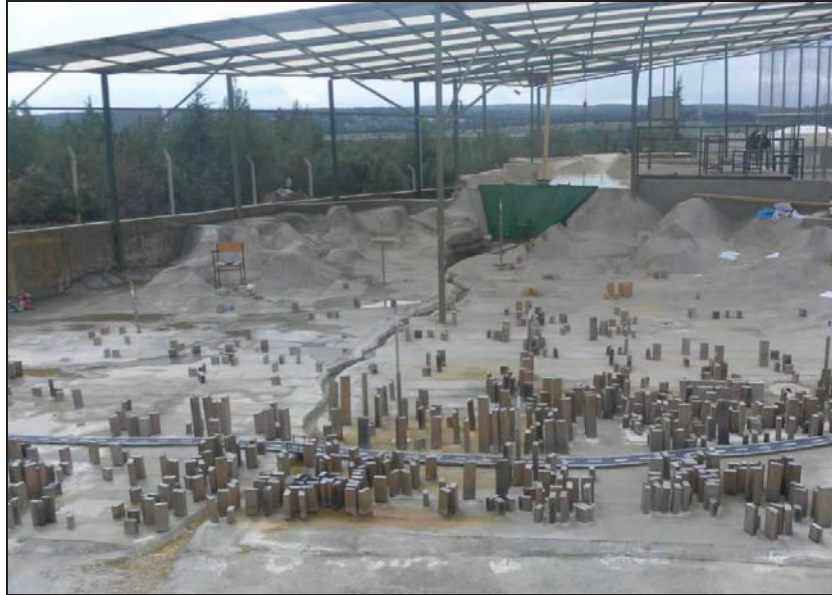
Figure 1. Physical model of Ürkmez Dam lake and downstream region without vegetation
