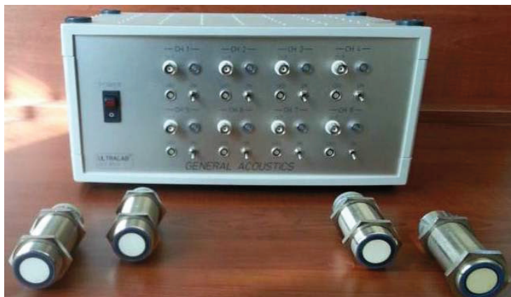
Figure 4. ULS 80D and USS20130 sensors.
