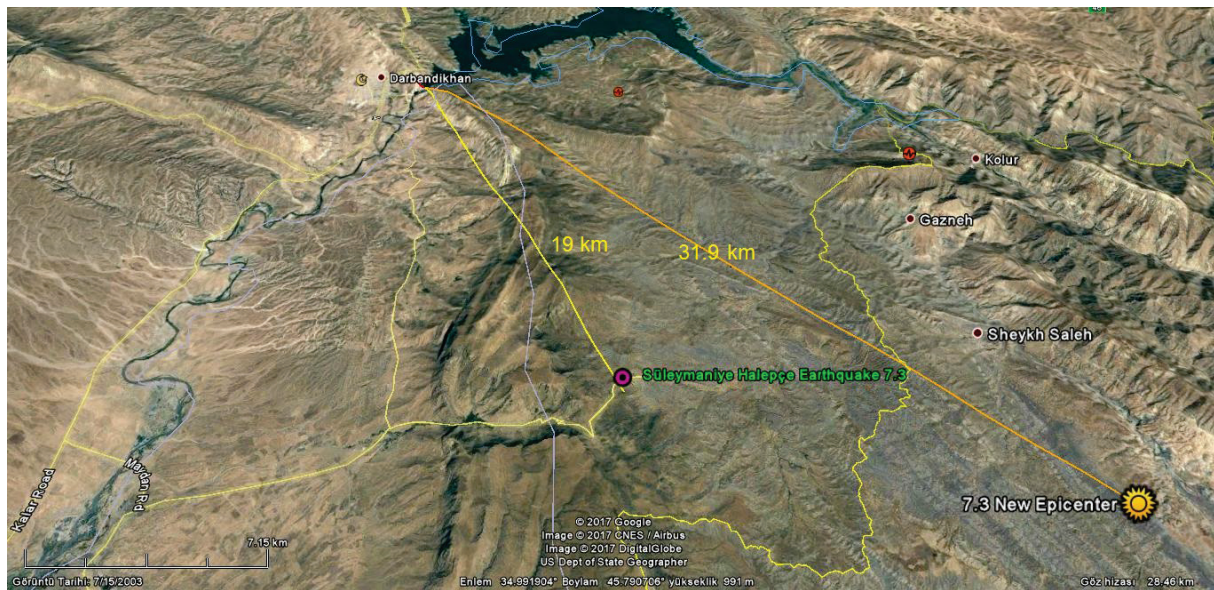
Figure 4. First and final epicenters announced and their distances with respect to Derbendikhan dam structure
