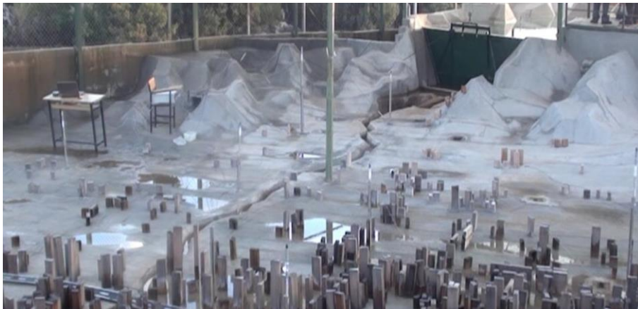
Figure 2. Distorted physical model of the Urkmez dam involving its reservoir and downstream part without any plant configuration
