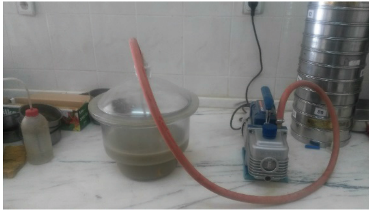
Figure 1. The saturation of core samples by using vacuum saturation equipment
