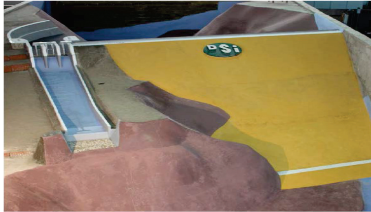
Figure 1. General overview of the 1/60-scaled physical model (Uyukluoglu, 2011)
