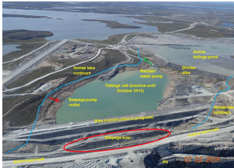
Figure 12. Tailings facility seepage area site plan
