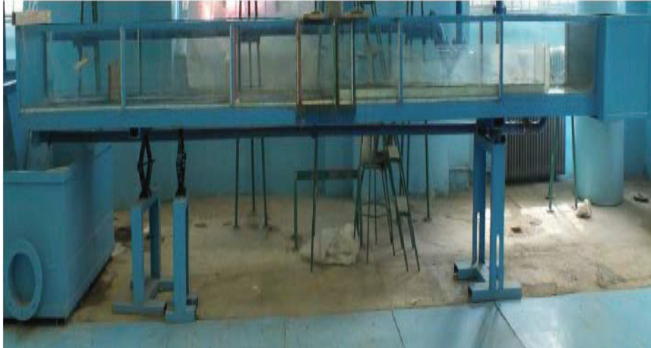
Figure 1. Dam break experiment using movable metal gate in a laboratory flume
