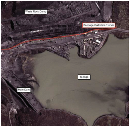
Figure 17. Tailings facility site plan
