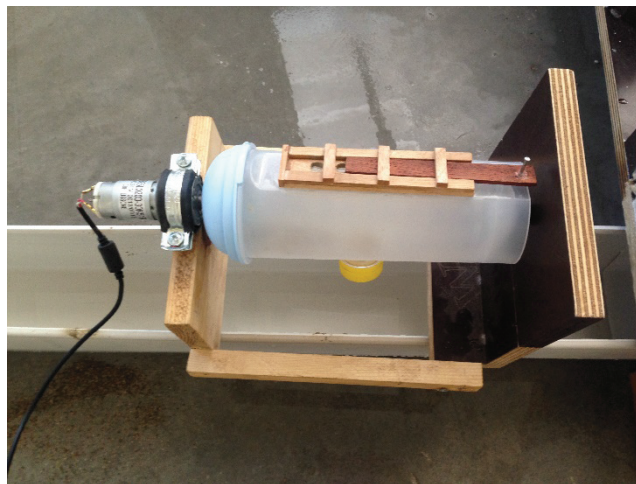
Figure 3. Sediment feeding system used in the experiments.
