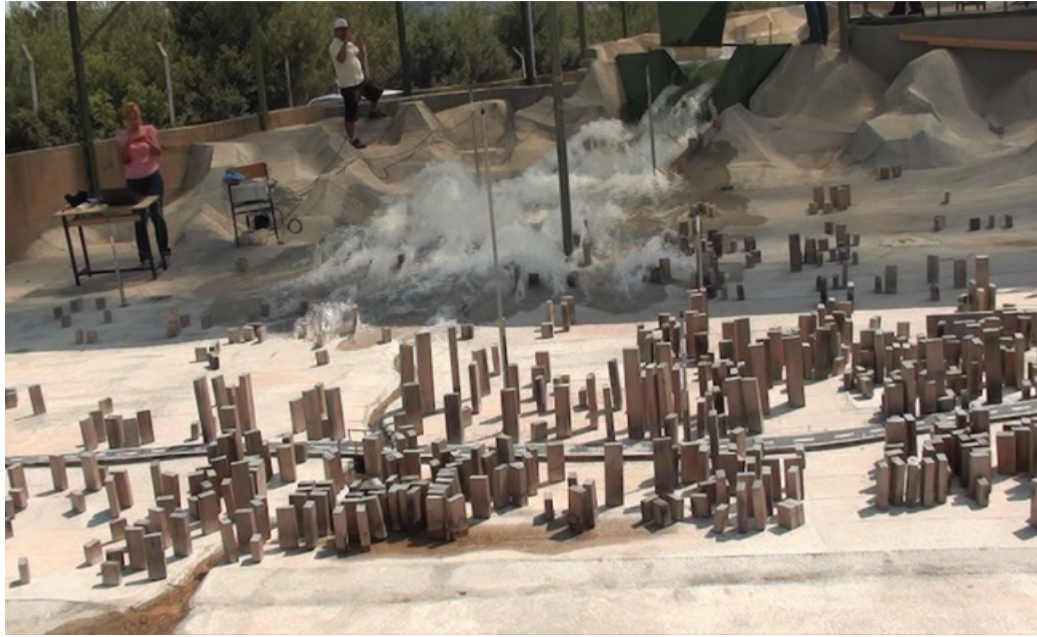
Figure 33. Dam break flood wave movement
