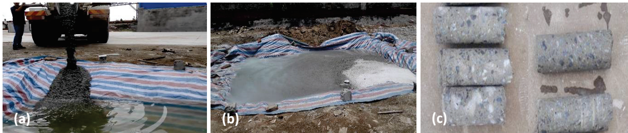
Figure 4. In-situ tests of SPUC including (a) pouring concrete, (b) complete pouring and (c) drill cores after hardening in the Tanjiang bridge project
