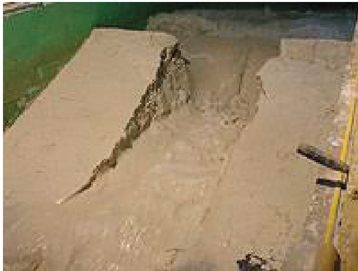
Figure 2. Gradual dam break experiment using compacted sand dam body in a laboratory flume
