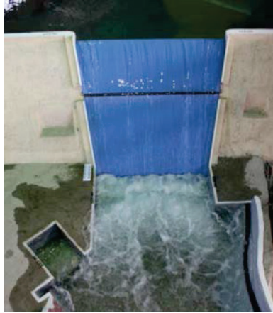
Figure 2. 1/60-scaled physical model with PMF discharge (Özcan, 2011)
